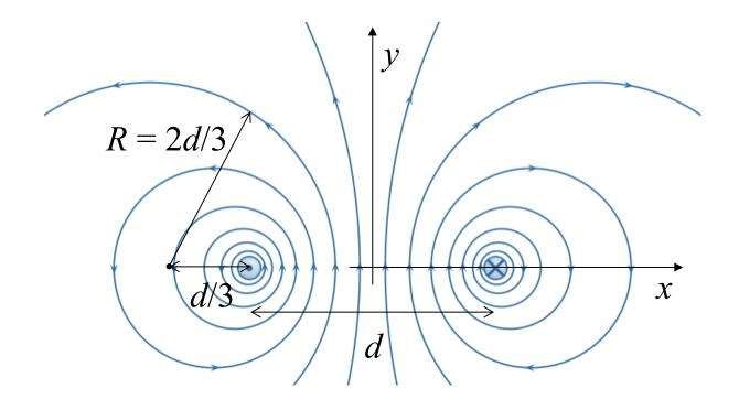
19. Refer to the diagram above – use Ampere's Law to determine the average field strength along the circle of radius R – compare to the geometric mean of the minimum and maximum that occurs along the circle.
