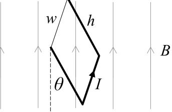
11. As shown below, a wire "U" with current 3.0 A is placed in a magnetic field  $\mathbf{B} =$ 0.015/x k, where B is in tesla and x is in meters. Determine the net magnetic force on the "U", each side of which is 3.0 cm.
