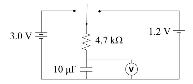
19. The capacitor in the circuit below is charged and discharged by closing and opening the switch. (a) Sketch voltage vs. time graphs for each resistor and the capacitor. Find the time constant for (b) discharging and (c) charging.
