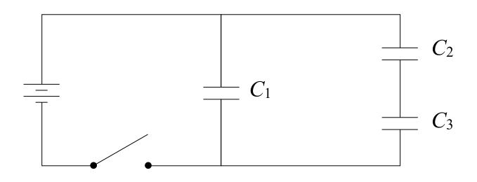
8. Capacitors  $C_1 = 4.7$  mF and  $C_2 = 1.2$  mF are connected to a 9.0 V battery as shown. Capacitor  $C_1$  is charged to 12 V as shown *before* the switch is closed. Find the eventual charge and voltage on each capacitor.
