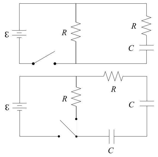
17. Resistors R<sub>1</sub> = 330 Ω and R<sub>2</sub> = 680 Ω, a capacitor C = 2.2 mF, and a 9.00 V battery are connected as shown. The switch is closed at t = 0 and then opened at t = 2.00 s. (a) Find the maximum voltage across the capacitor. (b) Make a careful sketch of voltage vs. time for each resistor and the capacitor.
