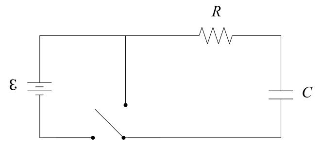
16. Make careful sketches of voltage vs. time and current vs. time for each capacitor charging and discharging. Determine the time constant for each action in terms of *R*, *C*, and relevant constants.
