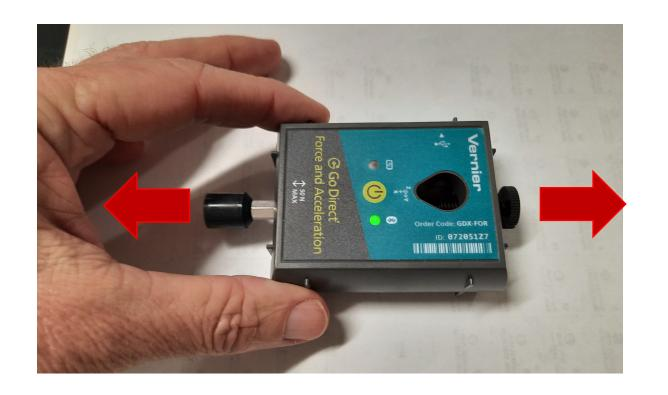
Without touching the force sensor, Collect data while rapidly sliding the device back and forth in the *x*-axis direction.
