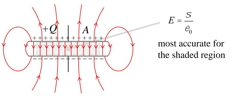
This expression applies *only* to the region *between* two oppositely charged surfaces separated by a relatively small gap. In reality the field weakens and curves near the edges of the plates and *outside* of the capacitor it is very weak and often assumed to be essentially nonexistent.
