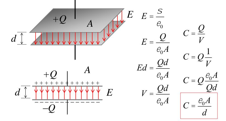
To derive capacitance in "terms of geometry" solve for the electric field and voltage for a given amount of charge. Then apply the basic definition of capacitance.
