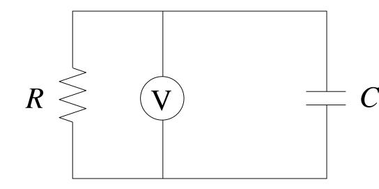
Collect data using a stopwatch. Use the "Lap" button to pause and unpause the total elapsed time displayed. The capacitor has been previously charged by a 6 V battery and will begin to discharge as soon as the circuit is completed.
