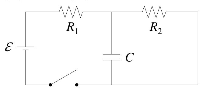
When the switch opens the time constant is  $R_2C$  as discharging occurs. However when the switch closes it is not obvious what happens! Sometimes it may be necessary to apply node and loop differential equations! It can be shown for this particular circuit that the time constant will be given by  $\tau = R_1R_2C/(R_1 + R_2)$  as charging occurs.
