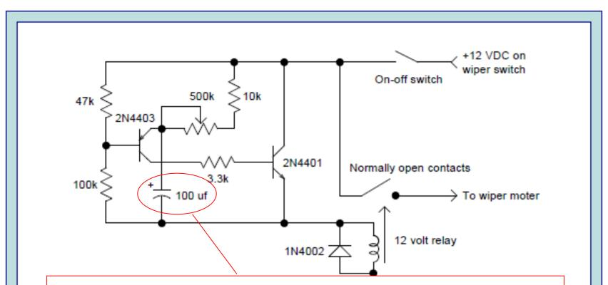
The wipers are turned on and off at a rate controlled and synchronized by the time it takes for the capacitor to charge and discharge. The time for this to happen can be adjusted with the variable 500 k $\Omega$  resistor. This is a good example of an application of an *RC* circuit. The capacitor in the circuit below is charged and discharged using the SPDT switch. Find expressions for voltage and current as functions of time.
