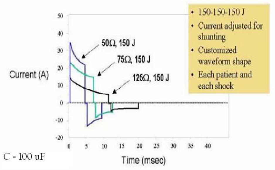
This is information for a defibrillator – essentially an *RC* circuit! The resistance is that of the patient's chest between the two paddles that are used to deliver the shock as the capacitor discharges.
