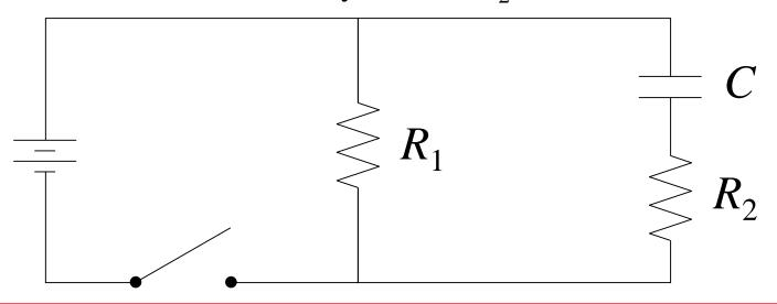
In principle any and every capacitor circuit problem can be solved by writing Kirchoff node and loop equations, substituting I = dq/dt, and solving the system of differential equations. However, there is often an easier way using only the notion of the time constant  $\tau = RC$  and appropriate exponential functions... (go to the next page to see)
