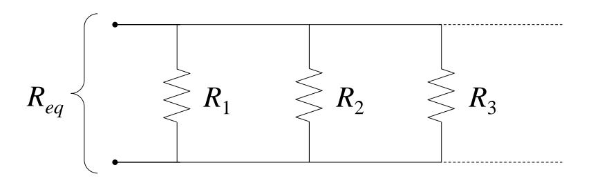
$$\frac{1}{R_{eq}} = \frac{1}{R_1} + \frac{1}{R_2} + \frac{1}{R_3} + \dots$$
