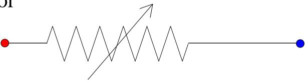
If only the blue and one of the red terminals are connected the device becomes simply a variable resistor that can be controlled by turning a knob or otherwise sliding the point of contact along the resistance wire.
