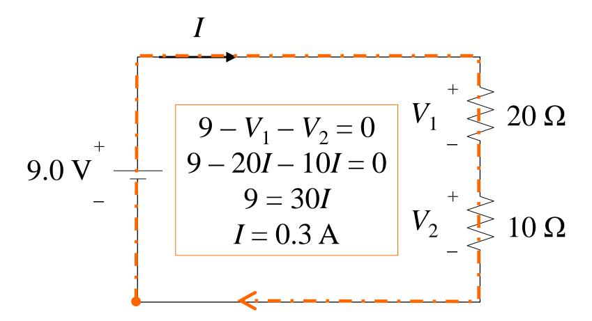
Following the green path counterclockwise around the circuit, the potential decreases by 9 volts and then goes up by amount *IR* for each resistor. This leads to a "loop equation" from which current can be determined with the same result.
