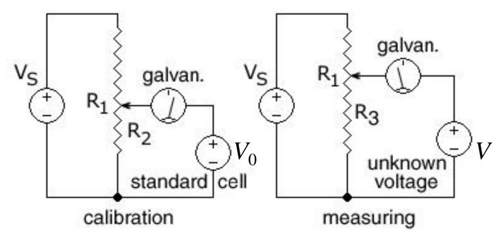
The sliding point of contact is adjusted until the galvanometer shows zero current. Using Kirchoff's Laws it can be shown that the unknown voltage V can is related to the standard cell by  $V = (R_3/R_2)V_0$ . The voltage  $V_S$  can be any amount. This circuit allows an unknown potential to be measured without any current through its source.
