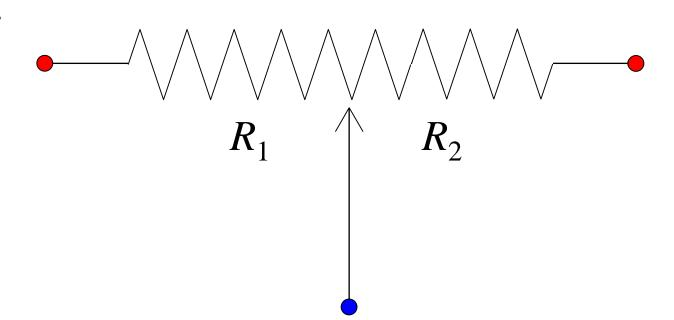
The total resistance  $(R_1 + R_2)$  between the two ends (red terminals) is constant. A certain part  $(R_1 \text{ or } R_2)$  of the total resistance exists between either end and the point of contact (blue terminal) depending on the length of wire between.
