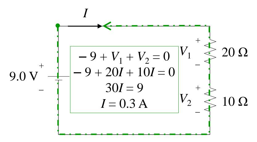
Here the direction of the current has been incorrectly drawn. *If* current *were* flowing thusly *all* of the voltages would be negative along of the blue path. Correctly analyzing the loop reveals that current must be in the opposite direction.
