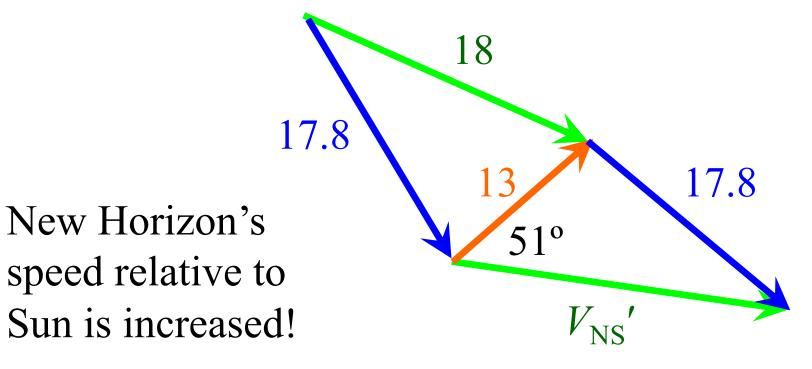
$$17.8^2 = V_{\text{NS}}'^2 + 13^2 - 2(V_{\text{NS}}')(13) \cos(51^\circ)$$
