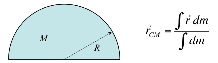
Find the center of mass of a semicircle of mass *M* and radius *R* cut from a thin uniform sheet (like a cutout).
