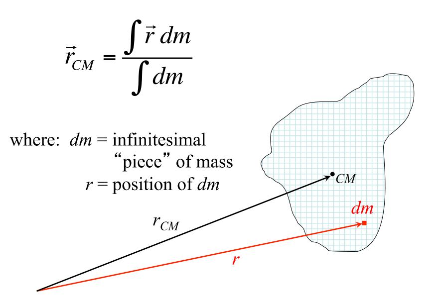
Example finding a center of mass using integration...
