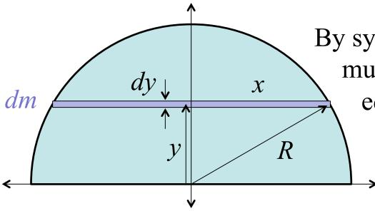
By symmetry the center of mass must lie on the *y*-axis. The equation of the circle is  $x^2 + y^2 = R^2$ .
