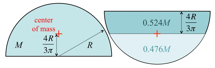
It is intuitively obvious that the center of mass is located on a *vertical* line of symmetry that divides the semicircle into two equal quarter circles of *equal* mass. But, don't get the wrong idea! A *horizontal* line passing through the center of mass does *not* divide the semicircle into two equal masses! A line through the center of mass and parallel to the diameter divides the mass into *unequal* parts 52.4% and 47.6% of the total.
