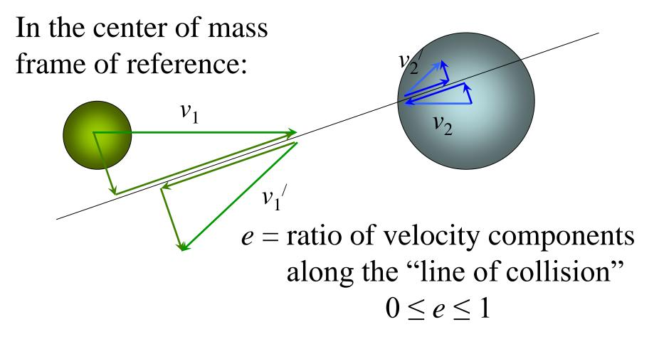
note: components perpendicular to this line are unchanged by the collision
