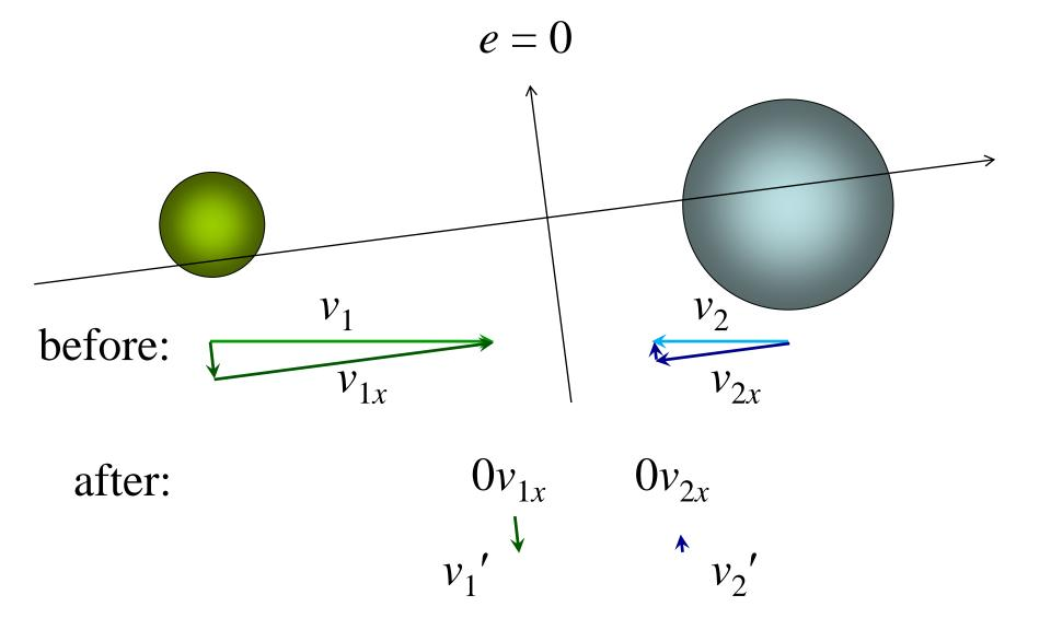
Use PhET Collision Lab to set this up and adjust "elasticity" – observe the effect on the components of the velocities. Compare also speed and kinetic energy and note that the percentage is not based on these quantities.
