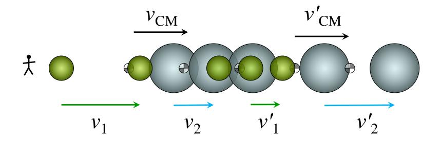
In this frame of reference the velocities and speeds of the two objects are different before and after the collision. But, what if the same collision were viewed in a frame of reference moving at the same velocity as the center of mass...
