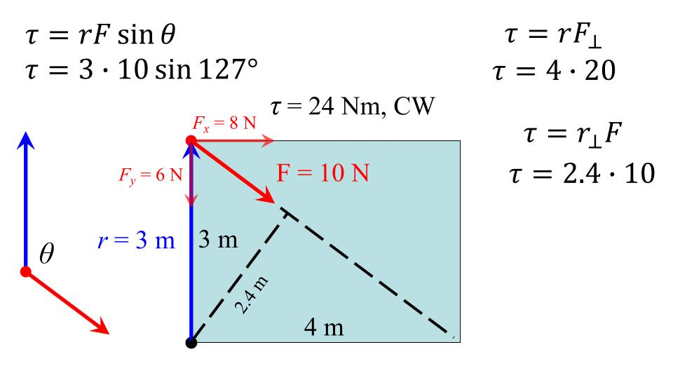
As shown in this example there are multiple approaches to determine the torque. Note that the perpendicular distance 2.4 m is an example of what is sometimes called a "moment arm", "torque arm", or "leverage arm".
