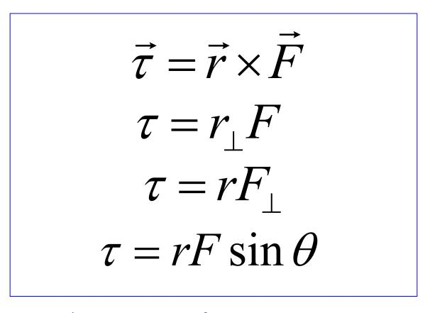
where: F = force r = position at which force is applied relative to axis of rotation.
