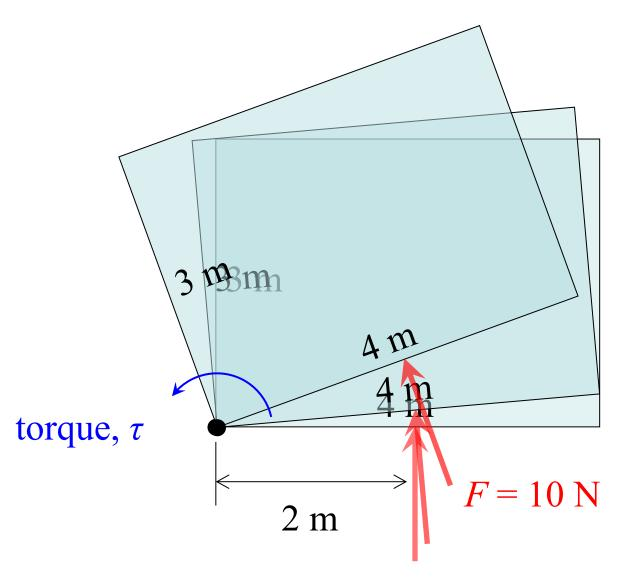
Torque quantifies "how effectively" a force causes angular acceleration. The same force applied at twice the distance from the axis causes twice the angular acceleration and constitutes twice the torque.
