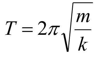
It is remarkable what is *not* in this equation – the amplitude or size of the oscillation. In other words the period <u>does not</u> depend on the size of the oscillations!
