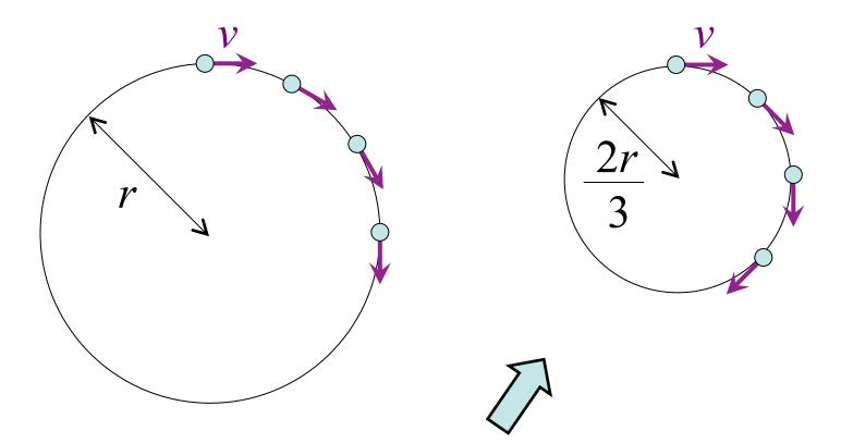
Moving at the same speed in a circle of two thirds the radius, an object changes direction a bit more rapidly would have 1.5 times the centripetal acceleration.
