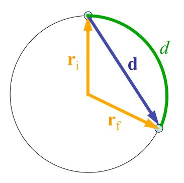
For *uniform* circular motion, speed may be found by simply dividing the distance by the time. The distance travelled in one *period* of time is the *circumference* of the circle. Therefore:
