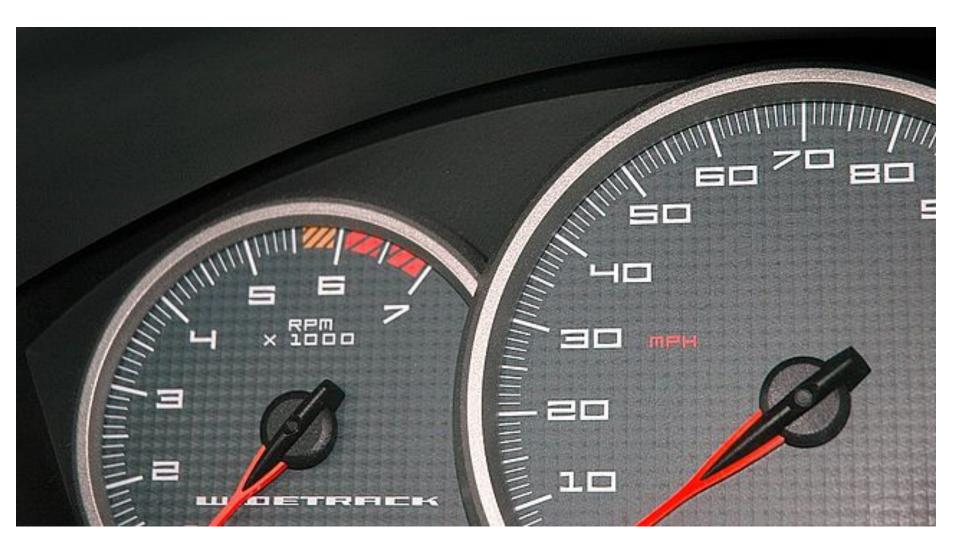
The tachometer indicates the frequency of the engine's crankshaft turning, measured in revolutions per minute.
