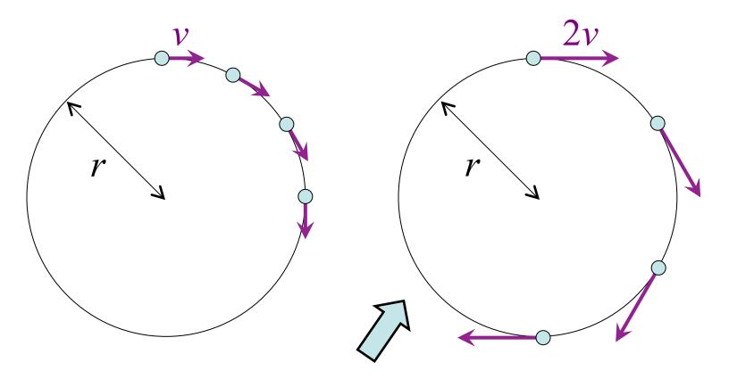
Moving at twice the speed in a circle of the same size, an object changes direction much more rapidly and would have 4 times the centripetal acceleration.
