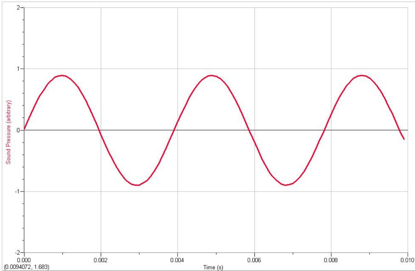
This is the output of an **oscilloscope**. An oscilloscope displays voltage vs. time – in this case the voltage output of a microphone.
