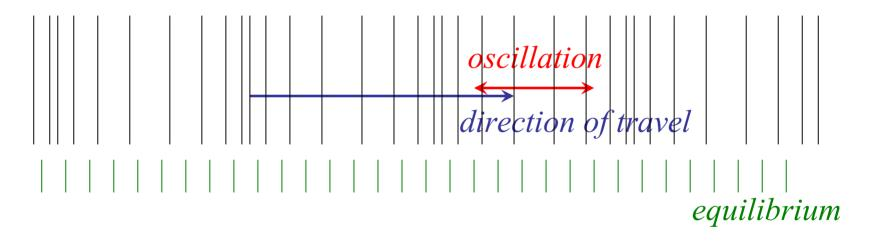
**Compression** = medium is more tightly spaced than normal
