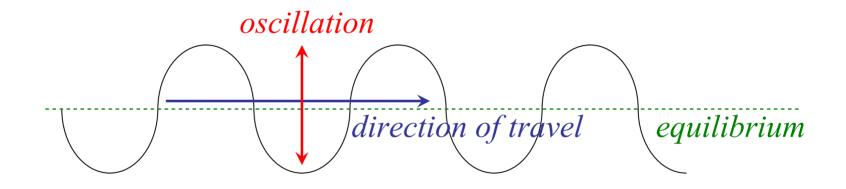
Crest = upward or positive displacement or change of the mediumTrough = downward or negative displacement or change of medium
