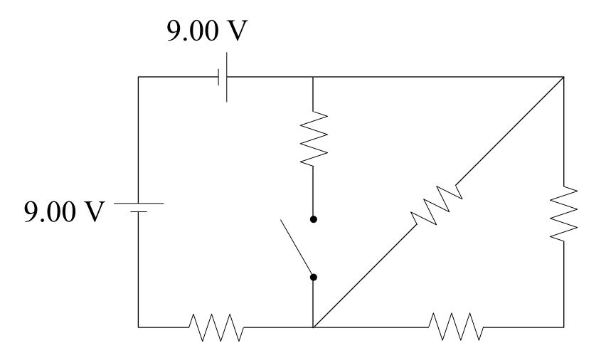
Each resistor in the circuit is  $10.0 \Omega$ . Determine the *change* in the power of the diagonal resistor when the switch is closed.
