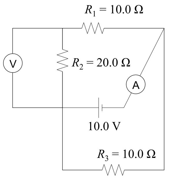
Determine the readings of each meter.
