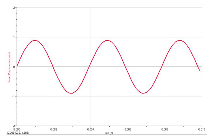
This is the output of an **oscilloscope**. An oscilloscope displays voltage vs. time – in this case the voltage output of a microphone.
