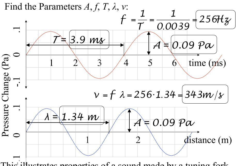
This' illustrates properties of a sound made by a tuning fork producing a sinusoidal pure tone near middle C on the piano.
