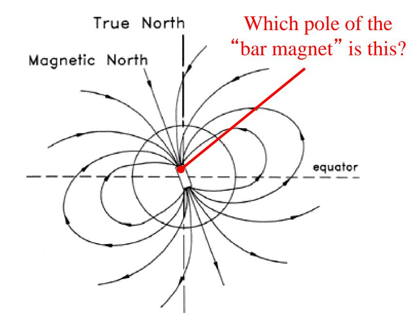
The Earth's *geographic* north pole behaves like a *magnetic* south pole! The magnetic north pole of a compass needle is attracted and so it rotates in that direction.
